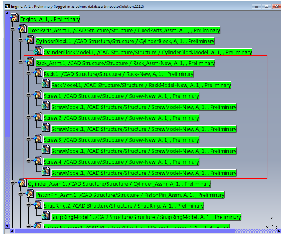
Picture 132: Existing PDM structure containing new substructure
