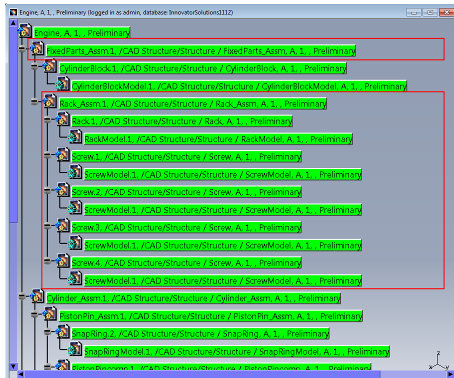
Picture 128: Existing PDM structure containing old substructure
